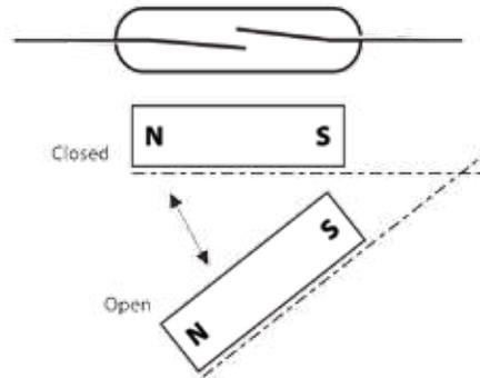
A pivoting/swinging magnet will operate the reed switch.
