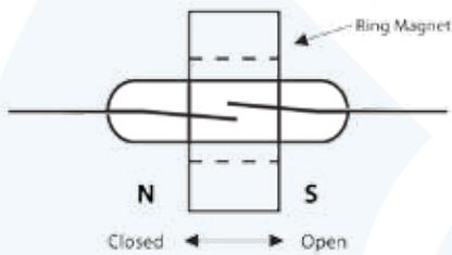
A reed switch moving through a circular/ring magnet will operate up to 3 times.
