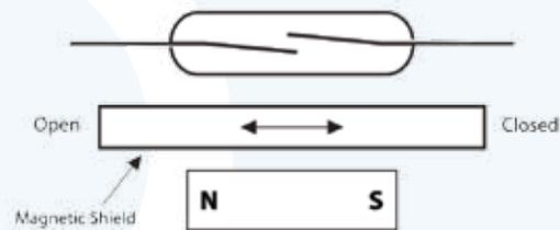
**Shielding (Indirect Actuation):**
