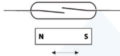
A reed switch can operate with a magnet moving parallel to the reed switch.
