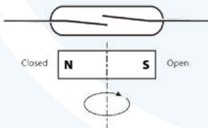
**Rotation:** Magnets can be rotated several different ways to operate the reed switch. For more information on the effects of rotary magnetic motions, contact HSI Sensing.
