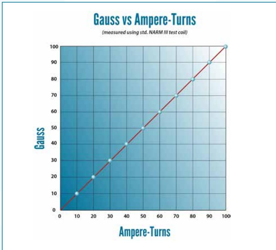
As a guide, approximately 0.1 milli-Tesla (mT) is equivalent to 1 Gauss is equivalent to 1 ampere turn. Many applications specify a specific magnetic field strength in Tesla, or more specifically mT.
